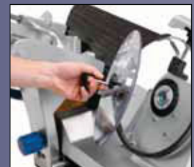
4: Remove Blade Safely
